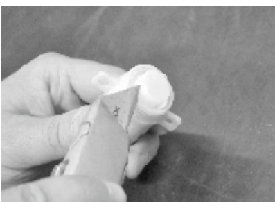
4. Taking out the turbine protection
