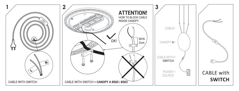
**WARNING!** THIS CABLE IS DESIGNED TO WORK ONLY WITH CAMELEON **CANOPY A 8565** | **8563** AND CAMELEON SHADES. THE FIXTURE MAY ONLY BE INSTALLED AND CONNECTED BY PERSONS QUALIFIED FOR WORK WITH ELECTRICAL EQUIPMENT.
